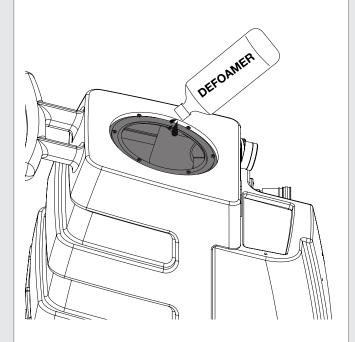
Add a defoamer in the recovery tank to reduce foam, prolonging the life of the Grand  $Prix^{TM}$  vacuum motor.
