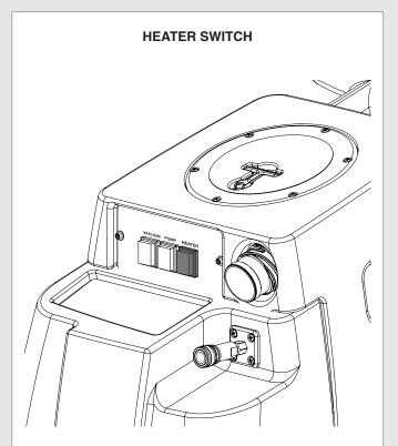
Release tool trigger. Turn on heater. Wait 8-10 minutes for unit to pre-heat. Once heated, re-key upholstery tool until hot water begins flowing. Once hot water is flowing, release trigger and pre-heat an additional 4-5 minutes.
