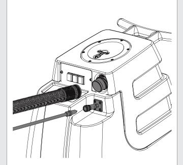
Attach one end of a solution hose to a wand or other tool, the other end to the Grand Prix™ front quick disconnect. Attach one end of a vacuum hose to the tool, the other end to the Grand Prix™ Cuff-Lynx™ vacuum hose port.
